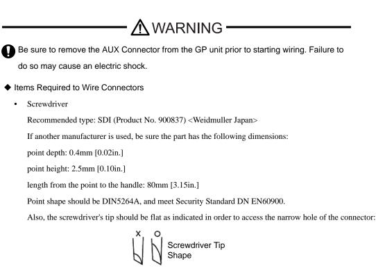
The connectors are a spring clamp type. Use the following procedure to connect the wires to the connectors.
