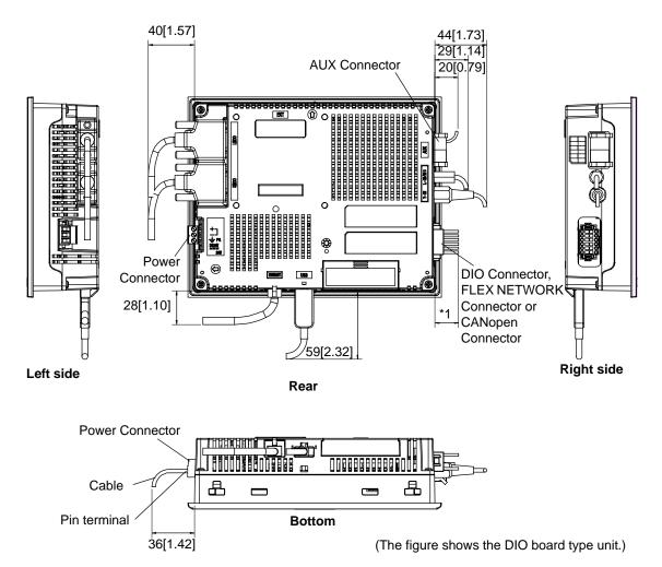
\*1 A 20 mm-space is necessary for the DIO/FLEX NETWORK board and a 127 mm-space for the CANopen board type.
