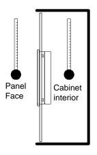
• Be sure that heat from surrounding equipment does not cause the GP to exceed its standard operating temperature. • When installing the GP in a slanted panel, the panel face should not incline more than 30°.
