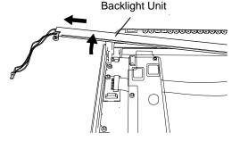
(8) Insert a new Backlight Unit while sliding it along the groove.
