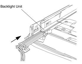
(10) Reattach the backlight unit's setscrew. The necessary torque is 0.196N•m.
