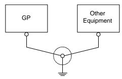
• When supplying power to the GP unit, be sure to separate the input/output and power lines, as shown. [diagram (a)]
