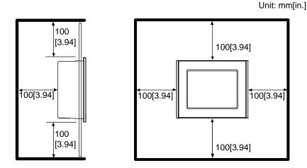
Be sure that the surrounding air temperature and the ambient humidity are within their designated ranges. (Surrounding air temperature: 0 to 50°C, Ambient humidity: 10 to 90%RH, Wet bulb temperature: 39°C max.) When installing the GP on the panel of a cabinet or enclosure, "Surrounding air temperature" indicates both the panel face and cabinet or enclosure's internal temperature.
