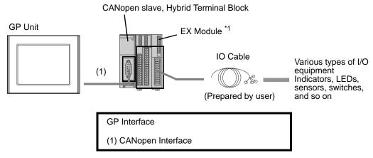
\*1 Up to seven EX modules can be connected to the CANopen slave, Hybrid Terminal Block.
