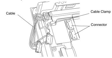
(7) Remove the hook from the Backlight Unit.
