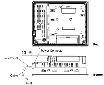
IMPORTANT • Depending on the type of connection cable used the dimensions shown above will change. The dimensions given here are representative values and are intended for reference only.
