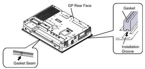
(4) Check that the gasket is attached correctly to the GP.
