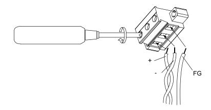
(6) Attach the Power Connector (Plug) to the GP and fix it to the GP main unit with right/left tightening screws.
