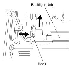
(8) Insert the new lower backlight unit into the backlight holder as shown here. After the backlight is completely inserted and the attachment clip clicks into place, lower the unit into the GP.
