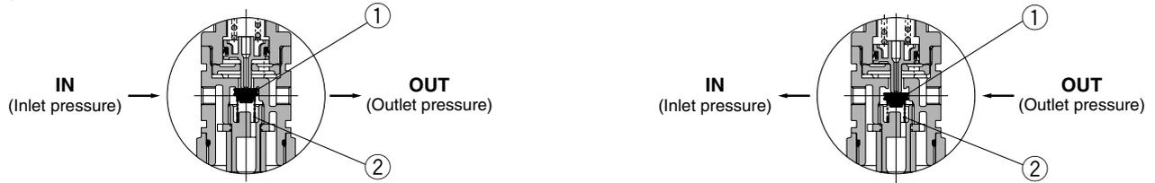
When the inlet pressure is higher than the regulating pressure, the check valve operates as a normal regulator (Figure 1).
